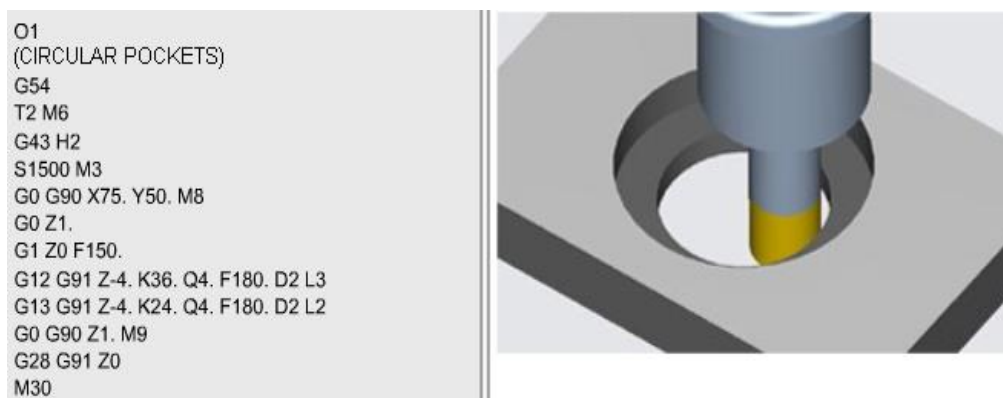
Figure 6. CN program and processing scheme.
