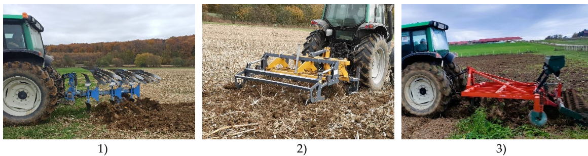
Figure 3. Display of attachment machines with which different soil treatments were performed: 1) plow (ST), 2) subsoiler (CTD) and 3) soil loosener (CTS).
