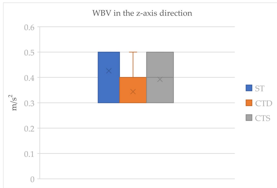
Figure 6. Boxplots of vibration with different tillage's in the z-axis direction.
