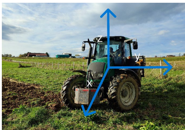
Figure 2. Display of the coordinate axes of the tractor during vibration measurement.
