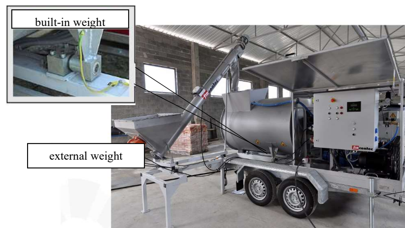
Figure 2. Special mixing machines to produce foamed concrete [73].
