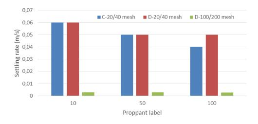
Fig 1. Settling rate of 20/40 and 100/200 mesh proppants in water.
