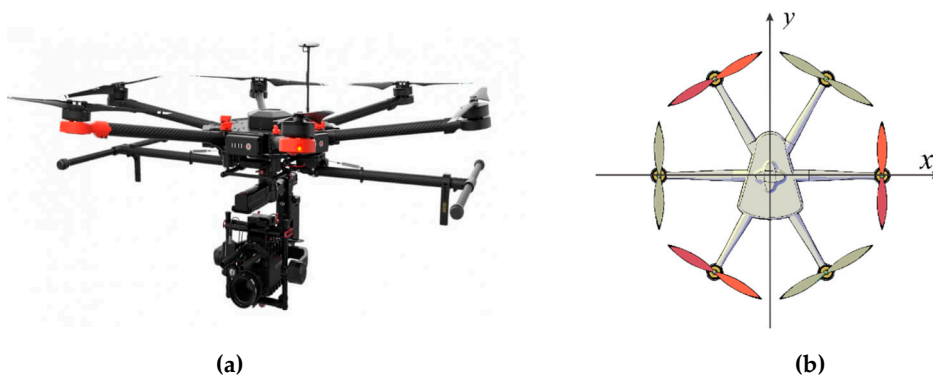
Figure 9. Hexacopter, (a) general view ; (b) motors' allocation.
