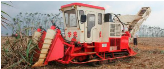
Figure 17. HN4GDL-91 sugarcane chopper harvester.
