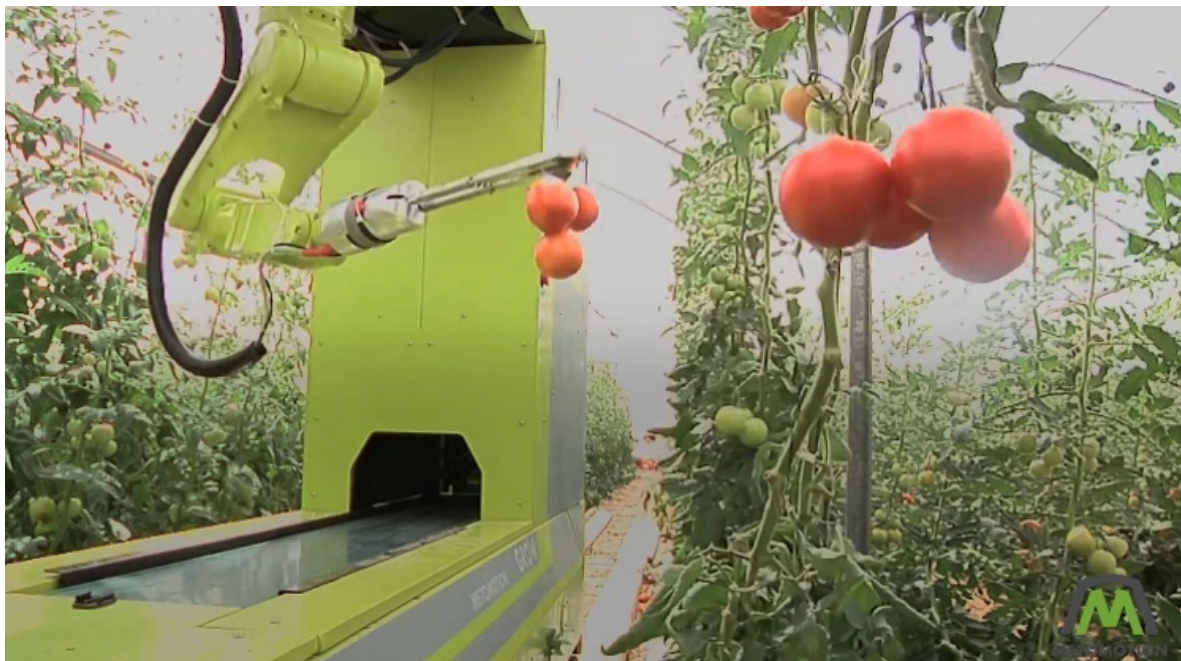
Figure 3. Figure 3 shows a robot in the process of harvesting, to achieve this it must have a very precise positioning system due to the difficult conditions of its environment.
