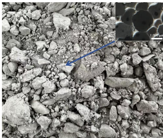
Figure 1. Waste foam concrete blocks obtained from construction waste dumping site.
