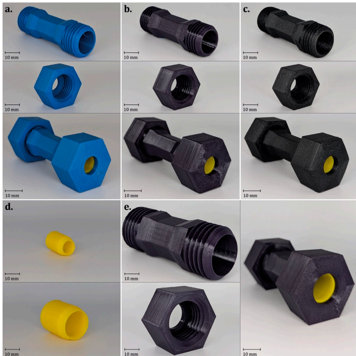
Figure 4. 3D printed pipe fitting parts for the test: (a) 10mm diameter pipe fitting parts made with PLA (from top to bottom: pipe fitting, nut, and assembled parts with the TPE gasket); (b) 10 mm diameter pipe fitting parts made with PETG (from top to bottom: pipe fitting, nut, and assembled parts with the TPE gasket); (c) 10 mm diameter pipe fittings made with ASA (from top to bottom: pipe fitting, nut, and assembled parts with the TPE gasket); (d) 10 mm (top) and 20 mm (bottom) gaskets made with TPE; and (e) 20 mm diameter fitting parts made with PETG (from top to bottom: pipe fitting, nut, and assembled parts with the TPE gasket).
