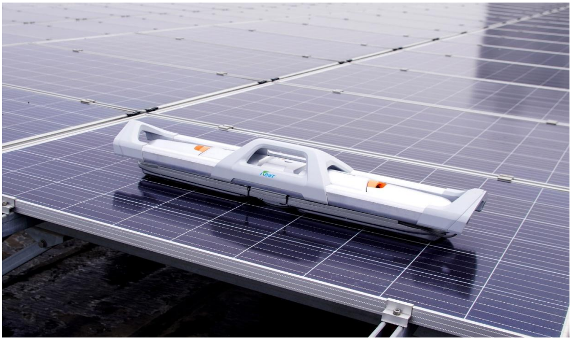
Figure 7. AI-powered robot called iFBOT for PV cleaning [16].
