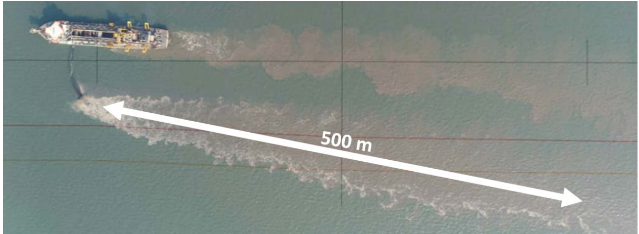
Figure 7. Lateral mixing of dredging plume.
