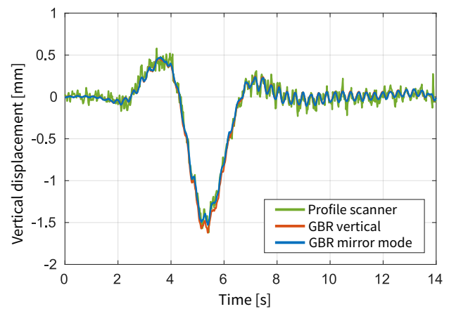
Figure 5 Comparison of the vertical displacement of the bridge for a truck passage measured with all sensors.
