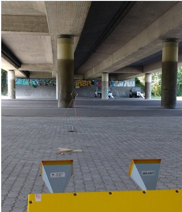
Figure 2 Setup of the GBR in mirror mode with a reflector under a concrete beam.
