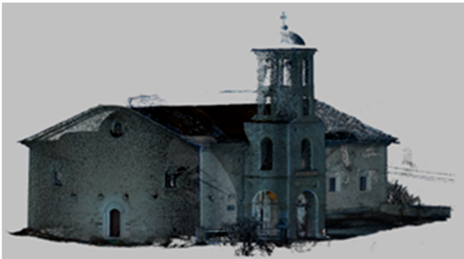
Figure 7. TLS-derived point cloud of the exterior of the Church of St. Petka.
