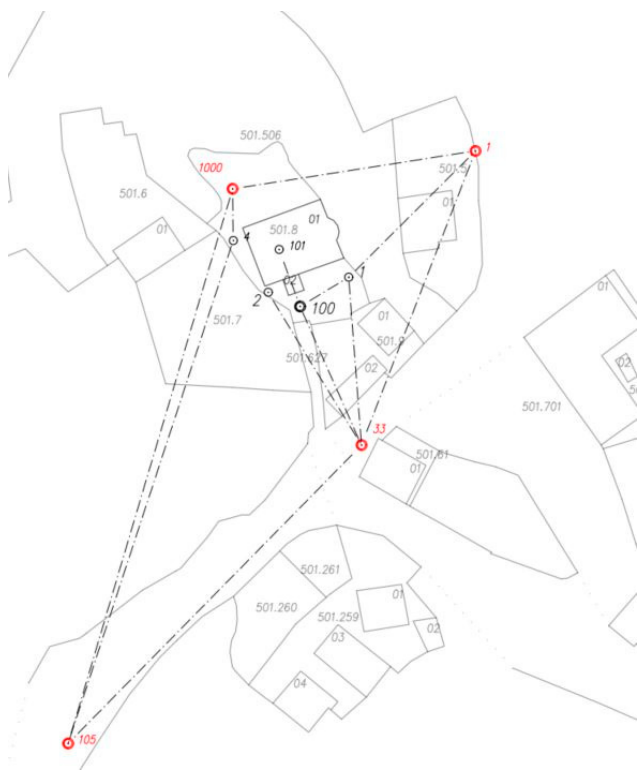
Figure 2. Spatial distribution of existing and newly established control points around and inside the Church of St. Petka.
