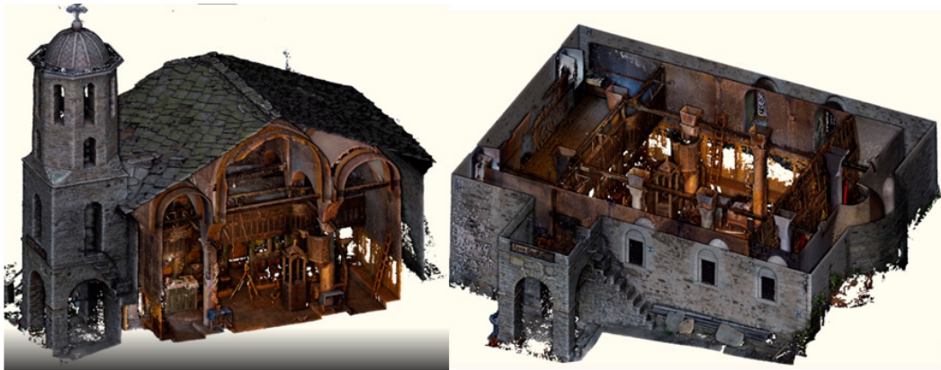
Figure 9. Point cloud obtained from UAV-based close-range photogrammetry.
