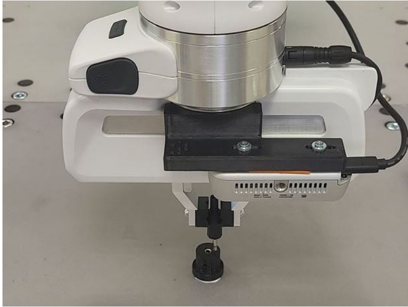
Figure 7. Experimental setup for testing the insertion of the audio pin into the socket.
