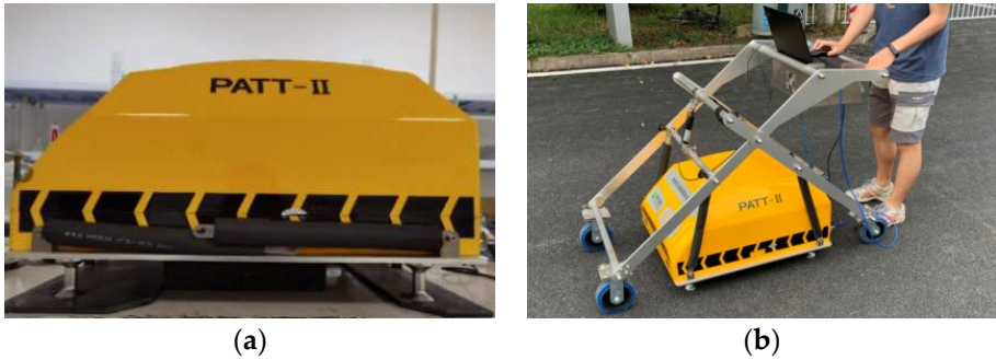
Figure 4. Pavement texture index test: (a) in-house testing,(b) Field testing.
