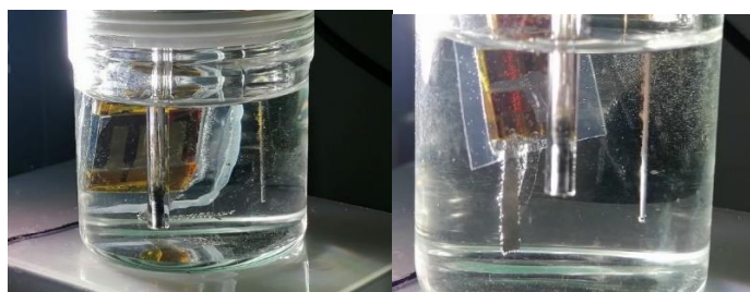
Figure 11. Magnified views of the perovskite-based photoanode showing the actual placement of the nickel electrodes on the Au terminals after encapsulation. (a) Configuration with a single Ni electrode placed on one Au pad of the device (b) Configuration with two Ni electrodes positioned on two separate Au pads, defining independent photoactive areas sharing a common ITO contact.
