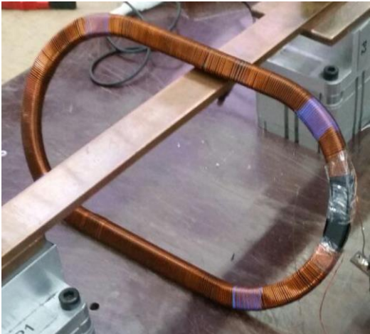
Figure 3. Case study: non-toroidal CT iron core and secondary winding manufactured.
