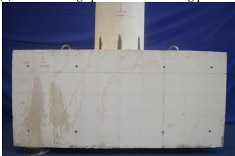
(c)Damage patterns on the south side of the bearing platform
