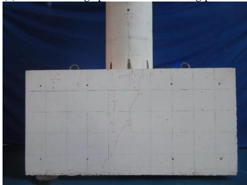
(c) Damage patterns on the south side of the bearing platform
