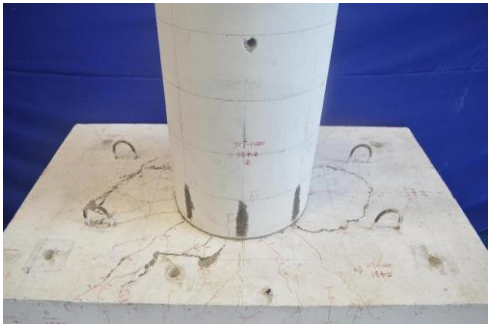
(a)Surface damage pattern of the bearing platform
