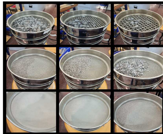
Figure 1. Gravel sieving after crushing test.
