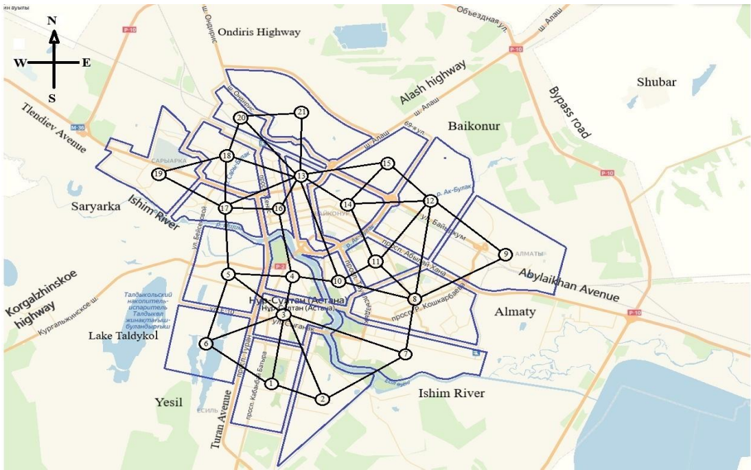
Figure 3. The adjacency structure of graph G of the core of a city model (using the city of Astana as an example).
