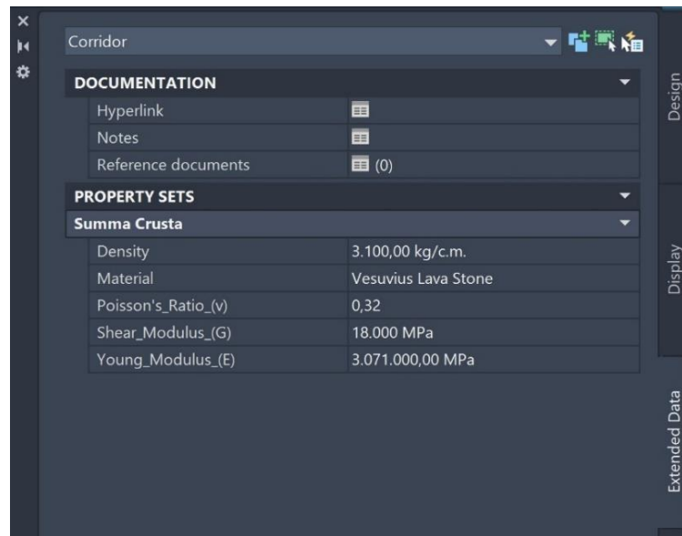
Figure 17. Property Set visualization in Corridor's Properties Extended Data Civil 3D section updated by means of Dynamo script.
