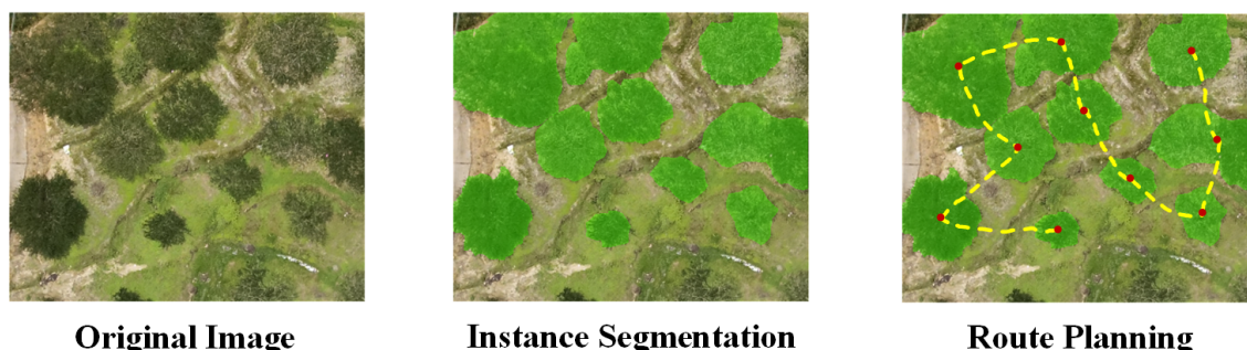
Figure 10. Flight path generation process. The drone uses a visible light sensor to acquire high-resolution images, and then inputs the images into the instance segmentation model for inference to obtain the segmentation masks; For each instance's segmentation mask, calculate its centroid as the target waypoint; Finally, optimal pesticide spraying flight paths are planned based on all the target waypoints.
