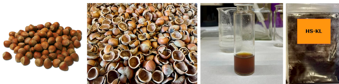
Figure 2. Steps of hazelnut shell processing from harvesting (a) to waste formation upon outer shell (HS) cracking (b), to lignin extraction from HS (HS-KL: Hazelnut-shell Klason lignin) (c), and finally to its powder upon vacuum drying (d).
