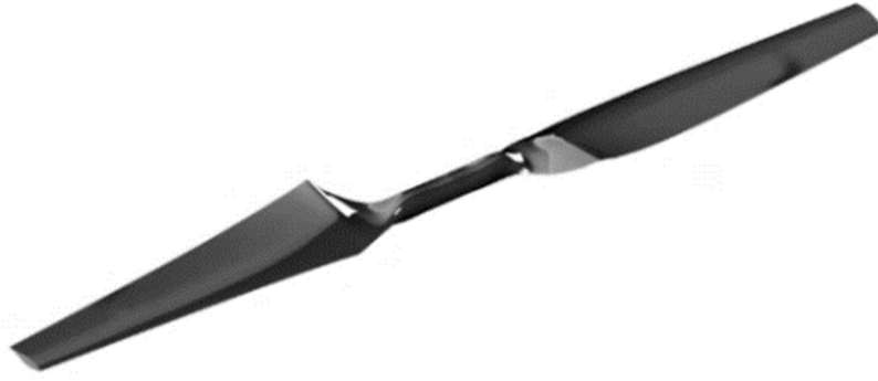
Figure 1. Shape model of the NREL Phase VI wind turbine blade.
