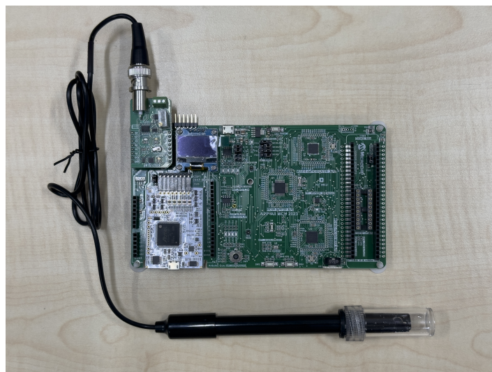
Figure 5. The final integrated device setup featuring the Microchip AVR128DA48 MCU, BME280, VEML7700, and pH sensor modules. The pH sensor is connected via a standard BNC cable for easy handling and calibration.
