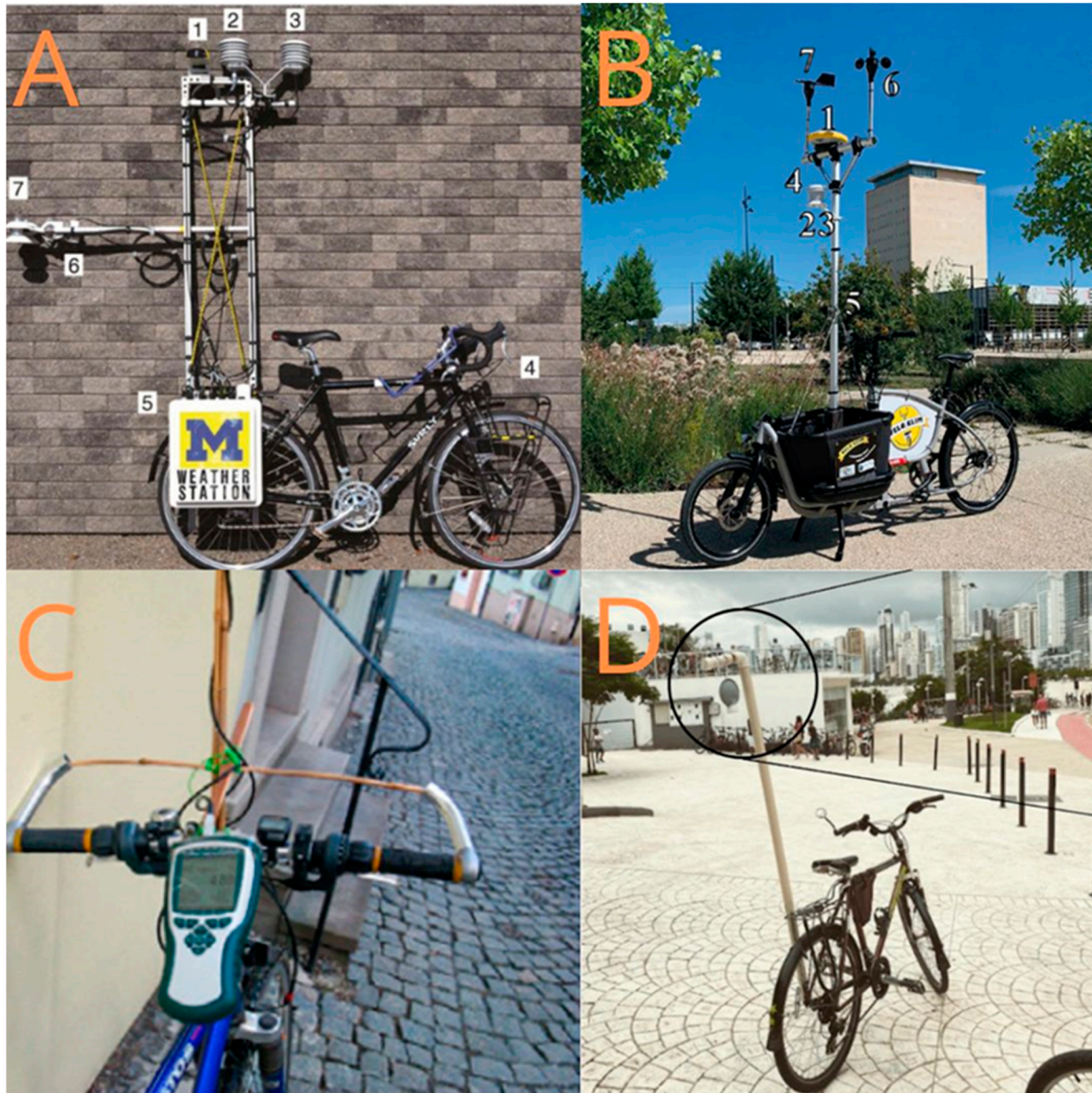
Figure 9. Equipment attached to bicycles for mobile measurements found in some of the selected articles. A) [8], B) [29], C) [27], D) [6]. Source: Authors (2023).
