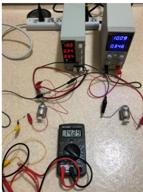
Figure 10-4. Experimental result when the initial input voltage is 10.0 V. The current meter reads I'_E > 14 A, much larger than the induced current I_{a0} (\approx 0.34 A). Even when the load is very large (1.0 M \Omega ), a substantially large current is flowing. Note that no Joule heating occurs in the motors, and a relatively large input voltage is allowed. That is, these motors can be repeatedly used even when the input voltage exceeds 3.0 V.
