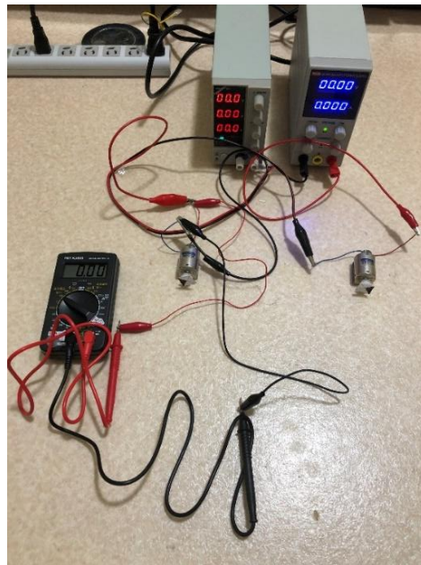
Figure 9-2. Experimental setup for measuring the emergent electric potential ( \varphi ). The voltage sources are two stabilized power supplies, one with a red light display; the other with a blue display. The two DC motors are not rotating at this time, as evidenced by the stationary black dots. The emergent electric potential is measured by a voltmeter (foreground).
