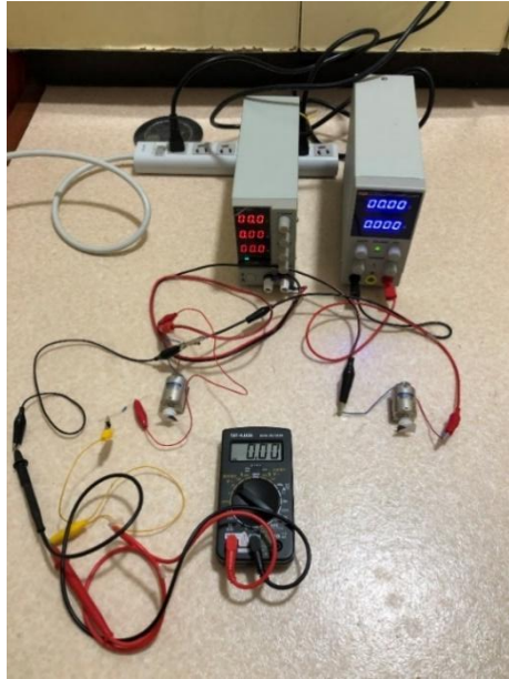
Figure 10-2. Initial setup of the experiment for harvesting the current ( I'_E ). Shown are the two voltage sources, the paired motors, a current meter (range 10 A), and a 1.0-M \Omega resistor connected by the red and yellow leads (in the vicinity of the left motor).
