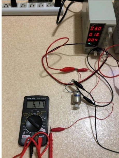
Figure 9-3. A result of the experimental setup in Figure 9-2. When the voltage source displays 3.0 V, the voltage associated with the emergent electric potential is 5.17 V, approximately 40% larger than the source voltage. From this result, it is evident that the current ( I_{a0} ) is induced current not ohmic one.
