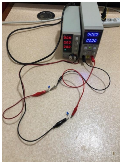
Figure 6-2. Initial setting of the experiment for confirming operation of the LED pair. The setup includes two power supplies (voltage sources) and two blue LEDs.
