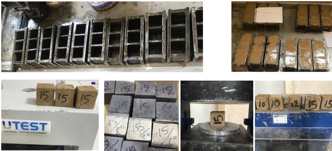
Figure 8. Stages of preparation, casting, and testing of the mortar mixes.
