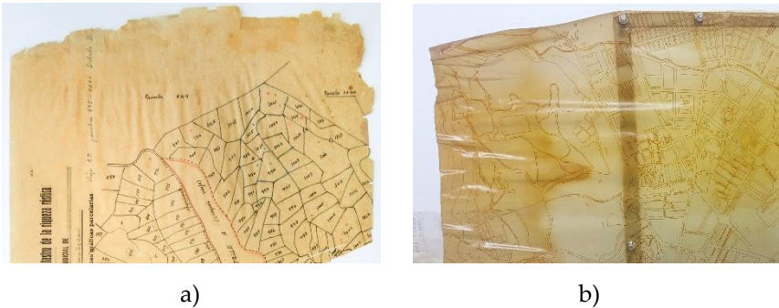
Figure 3. Comparison of surface texture: (a) document without emulsion or surface preparation corresponding to group T3G2 in Table 3 (image of document AHP729); (b) document with intaglio emulsion corresponding to group T3G3 in Table 3 (image of document ETSAGG12).
