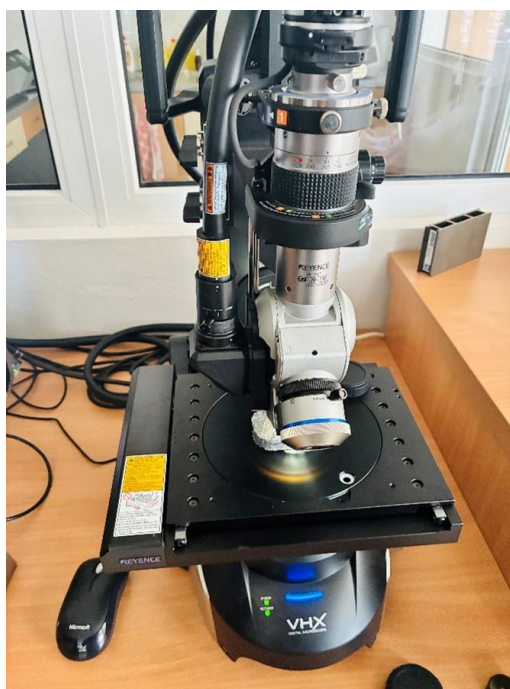
Figure 3. Keyence VHX-6000 digital microscope used for 3D surface analysis of the pressed briquettes.
