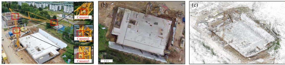
Figure 8. Schematic diagrams of the experimental site: (a) the experimental site and the layout of surveillance cameras; (b) the digital orthophoto map of the experimental site; (c) the sparse point cloud of the experimental site obtained through oblique photography and SfM reconstruction.
