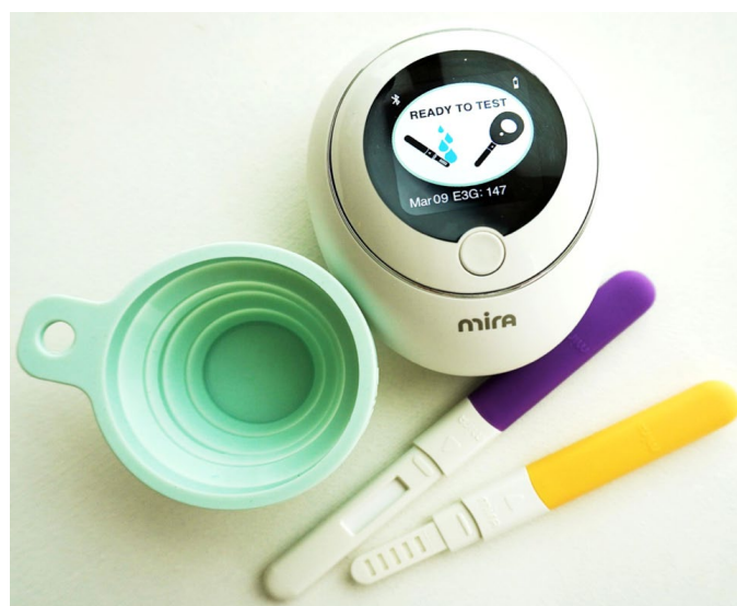
Figure 1. Mira Monitor with urine test sticks and sampling cup. Test sticks are inserted into first-morning urine in the sampling cup for 20 seconds before inserting into the monitor to be analyzed.
