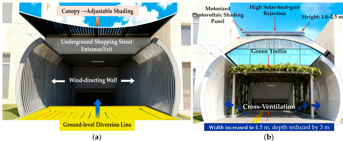
Figure 16. Optimization of entrance and exit shapes for airflow enhancement. (a) Motorized PV canopy plus curved walls widen shortened entry for airflow. (b) Reflective ground lines channel wind through expanded entrance, boosting ventilation.
