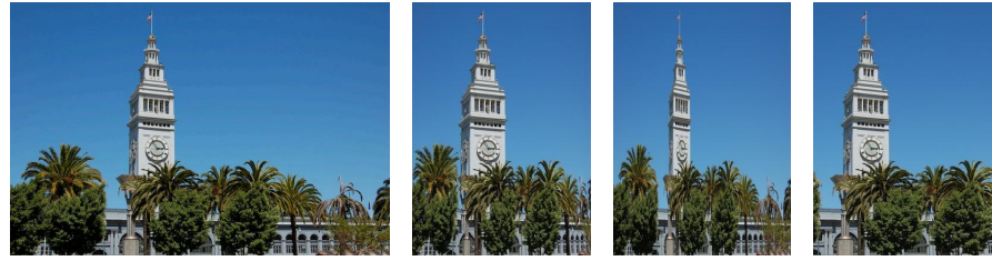
Figure 3. From left to right, original image, its retargeting results with seam carving, scaling and cropping respectively[119].
