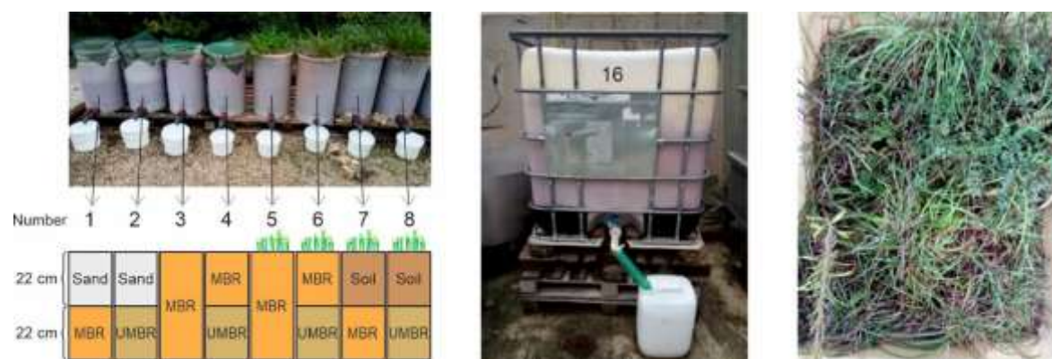
Figure 1. Lysimeters experimental setup. Left: 40-L lysimeters, view and diagram of filling and revegetation; center and right: 700-L lysimeter, shown from the side and from above, respectively.
