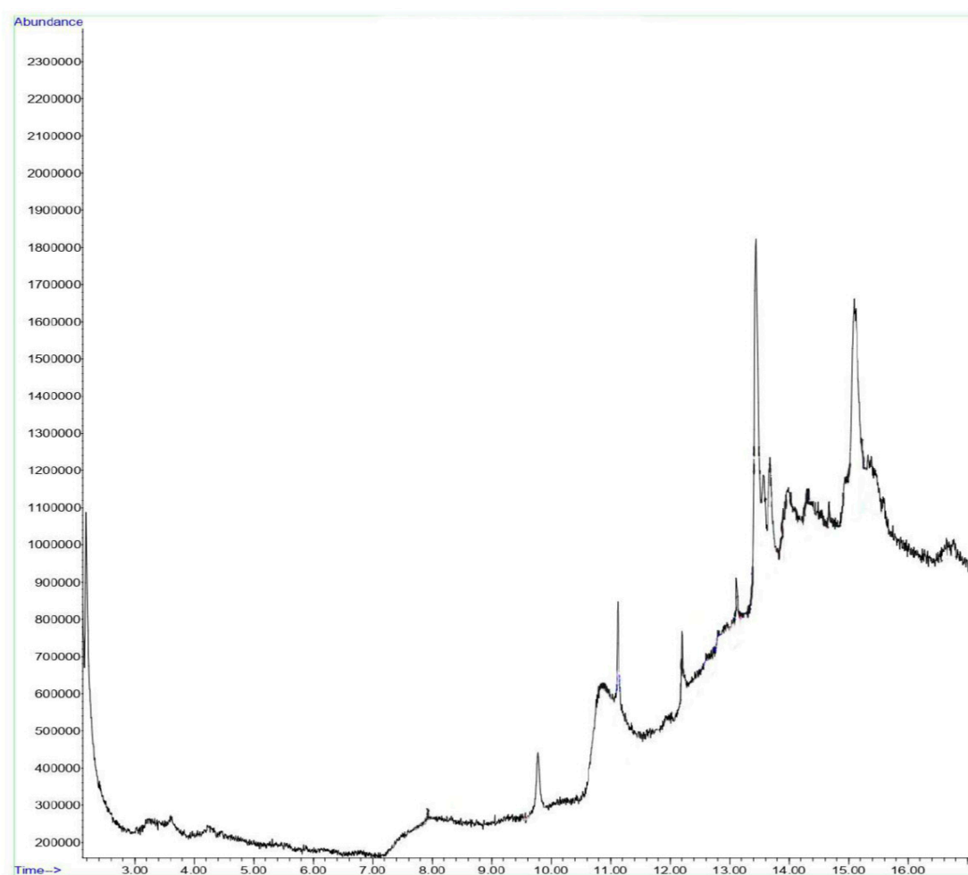
Figure 1. GCMS spectrum of APMLE showing abundances of bioactives present and the retention time.
