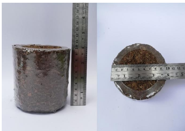
Figure 2. Cylinder shape leaves waste planting blocks 10 cm in diameter and 10 cm high.
