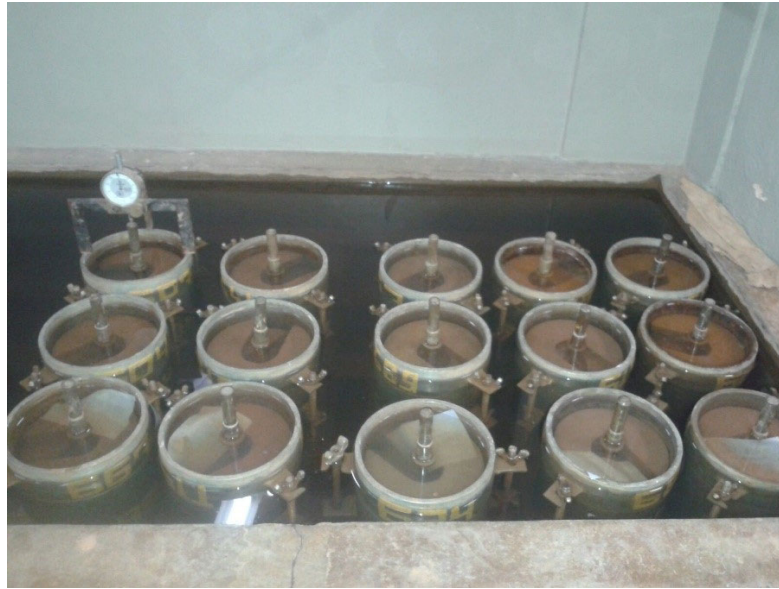
Figure 1. Submerged specimens to determine the expansion and CBR later.
