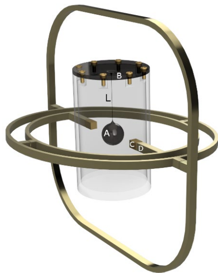
Figure 3. Pendulum-based seismometer mounting design. A: pendulum bob; B: rim of the housing’s top lid. C: housing mounting pivot; D: three-ring gimbal mounting pivo; L: pendulum length.
