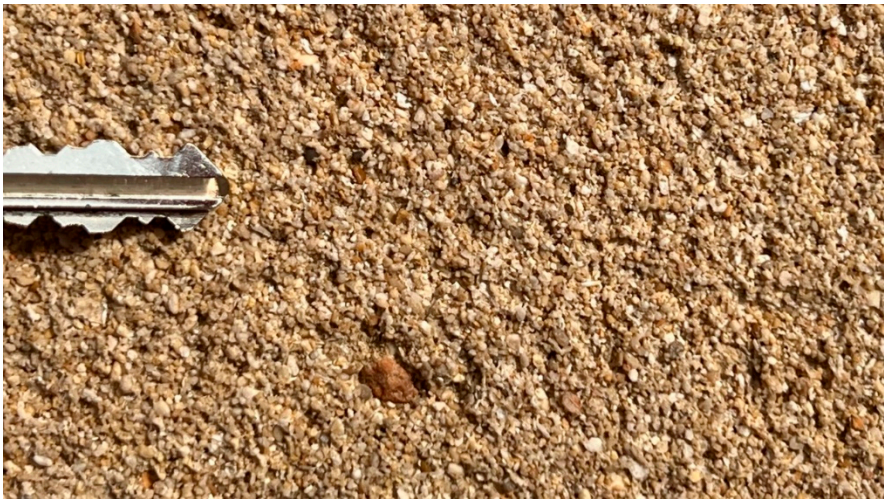
Figure 4. Detail of a marés sandstone sample showing its porous texture and granulometric variability. The key provides an approximate scale. The open structure is characteristic of marés sandstone from coastal quarries (photograph by the author).
