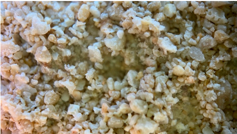
Figure 5. Enlarged image of an ashlar captured with a digital loupe. Rounded bioclastic grains, poor cementation, and interconnected channels are visible, all of which promote capillary action and moisture retention (photograph by the author).
