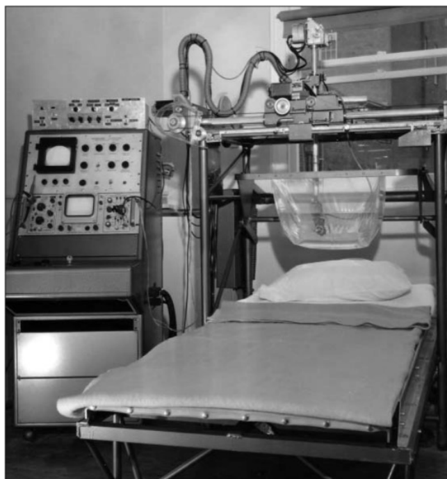
Figure 3. An early ABUS system designed by George Kossof and Jack Jellins in Australia, showing the enclosed water bath that was lowered across the patient's chest [16]. The ultrasound transducer can be seen in the water bath. © American Institute of Ultrasound in Medicine.
