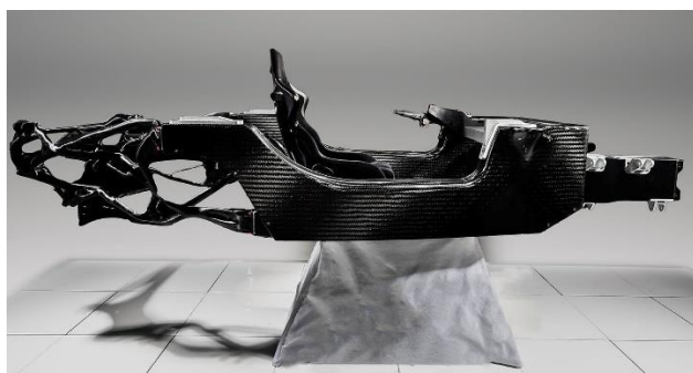
Figure 1. F1 chassis made of Carbon-fibre-reinforced-polymer (CFRP) [source: THEDRIVE].
