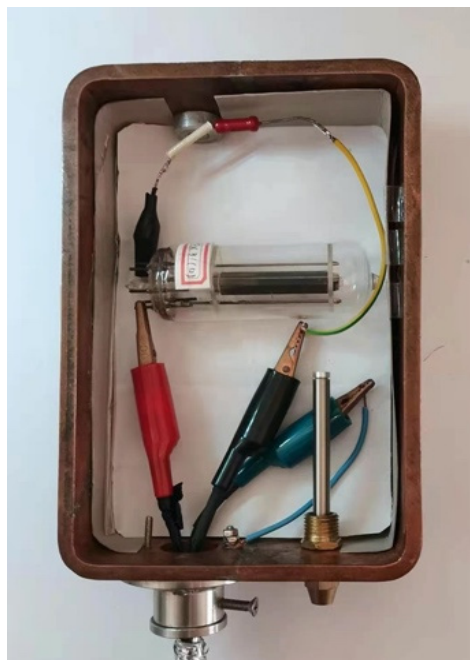
(2) The interior of the copper shielding box
