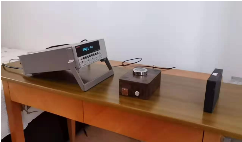
Keithley 6514 ( 10^{-16} A) copper shielding box magnet (1) The set up of the experiment
