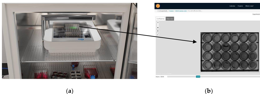
Figure 1. The cloud-based Omni device: (a) the device inside the laboratory incubator; (b) Online adjustable view of ongoing experiments (cells in well plates), including real-time analysis capabilities.
