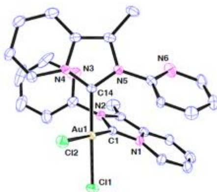
Figure 9. ORTEP view of 3 (30% probability). The H, \text{PF}_6 , and \text{H}_2\text{O} species have been omitted for the sake of clarity. Pertinent bond lengths (angstroms) and angles (degrees): \text{Au}(1)\text{--C}(1) = 1.996(6) , \text{Au}(1)\text{--C}(14) = 2.014(5) , \text{Au}(1)\text{--Cl}(1) = 2.2984(16) , \text{Au}(1)\text{--Cl}(2) = 2.3150(16) , \text{N}(1)\text{--C}(1) = 1.360(7) , \text{N}(2)\text{--C}(1) = 1.363(8) , \text{C}(14)\text{--N}(4) = 1.338(7) , \text{C}(14)\text{--N}(5) = 1.347(7) , \text{N}(1)\text{--C}(1)\text{--N}(2) = 105.3(5) , \text{N}(4)\text{--C}(14)\text{--C}(5) = 106.2(4) , \text{C}(1)\text{--Au}(1)\text{--C}(14) = 89.9(2) , \text{C}(1)\text{--Au}(1)\text{--Cl}(1) = 88.08(17) , \text{C}(14)\text{--Au}(1)\text{--Cl}(1) = 177.89(15) , \text{C}(1)\text{--Au}(1)\text{--Cl}(2) = 177.91(17) , \text{C}(14)\text{--Au}(1)\text{--Cl}(2) = 90.22(16) , and \text{Cl}(1)\text{--Au}(1)\text{--Cl}(2) = 91.86(7) . [104].
