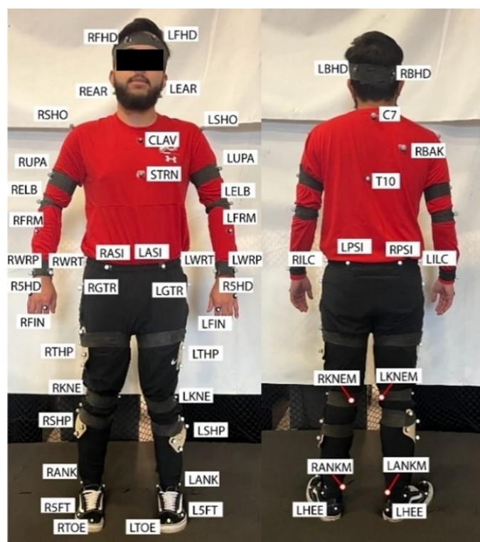
Figure 2. Motion Capture Marker Setup [23,24].
