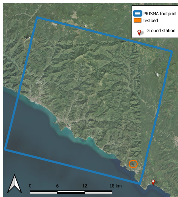
Figure 7. Geographic extent of the second testbed (Monterosso, in Northern Italy), highlighting PRISMA coverage (tilted blue square), the chosen testbed area simultaneously acquired by both Sentinel-1 and PRISMA (small orange square in an orange circle at the bottom-right corner of the PRISMA coverage) and the ground-truth station (red dot at the bottom-right corner of the Figure, outside the PRISMA coverage area).
