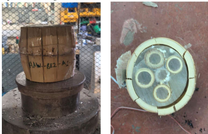
Figure 5. Image of a stocky HAW-BE2-M-ST specimen.
