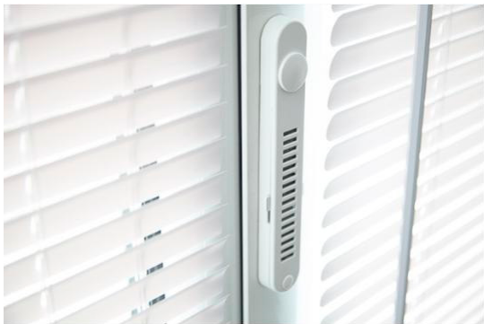
Figure 6. Prototype of the window-integrated air purification system installed on a window with blinds.
