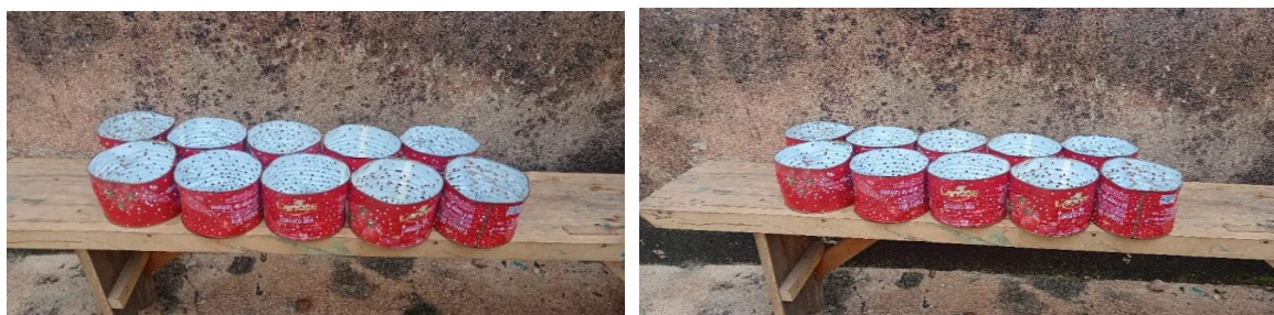
Figure 3. Perforated tin tomato cans as reaction vessels for the synthesis of pectinase.
